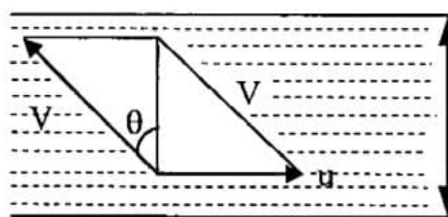
$$\therefore \sqrt{v^2 - u^2} \times 5 = 100 \Rightarrow v^2 - u^2 = (20)^2 \Rightarrow (25)^2 - u^2 = 400 \quad \therefore u = 15 \text{ m/min} \quad (\text{Ans.})$$
