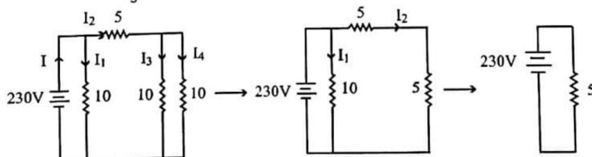
$$\text{চিত্র হতে, } I_2 = \frac{10}{20} \times 46 = 23 \text{ Amp} \text{ এবং, } I_4 = \frac{10}{20} \times 23 = 11.5 \text{ Amp}$$
