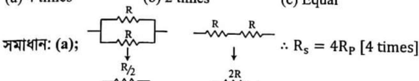
03. What is the equivalent resistance of the circuits if each has a resistance of  $600\ \Omega$ ?
