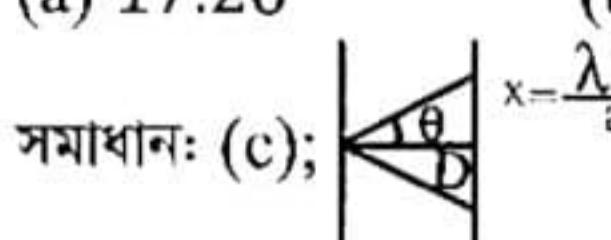
$\sin\theta \Rightarrow \frac{x}{D} = \frac{\lambda D}{a} = \frac{\lambda}{a} = \frac{5.896 \times 10^{-7}}{4 \times 10^{-6}}$ ;  $\theta = 8.48^\circ \therefore 2\theta = 16.95^\circ$
