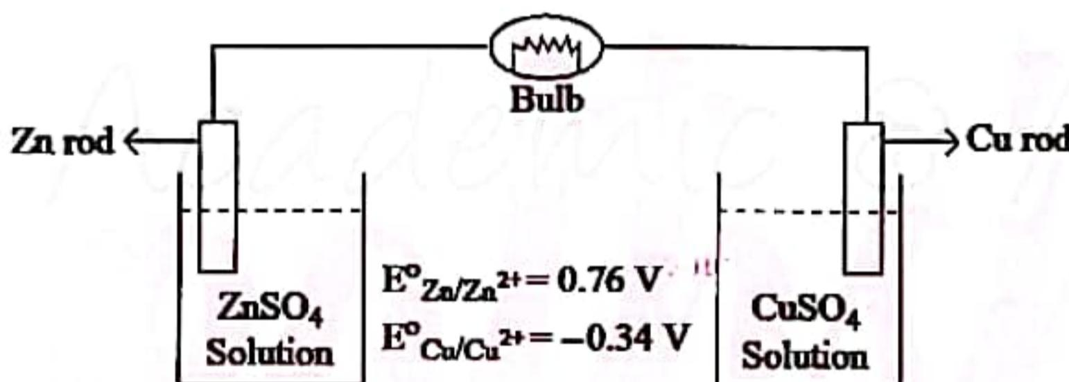
$$\text{সমাধান: } V = E^\circ = E^\circ_{\text{Zn}/\text{Zn}^{2+}} + E^\circ_{\text{Cu}^{2+}/\text{Cu}} = 0.76 + 0.34 = 1.1 \text{ V}$$
