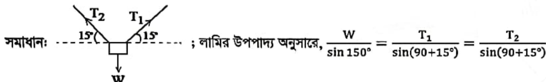
$$\Rightarrow T_1 = \frac{W}{\sin 150^\circ} \times \cos 15^\circ = 851.9465 \text{ N}; T_2 = 851.9465 \text{ N}$$
