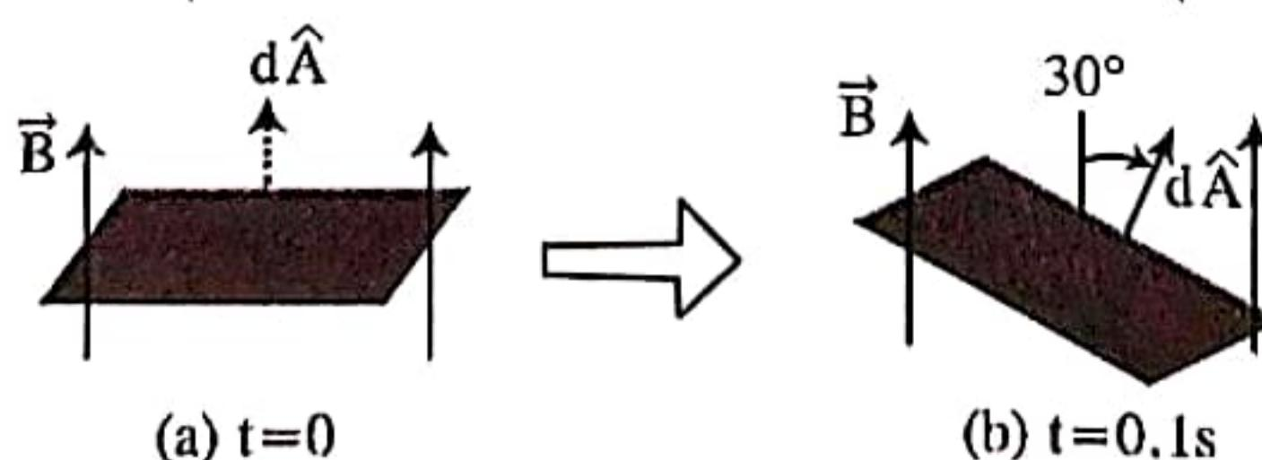
$$\text{সমাধান: } \epsilon(+) = \frac{d}{dt} \phi = \frac{d}{dt} \vec{A} \cdot \vec{B} = \frac{d}{dt} AB \cos \theta = A \frac{d}{dt} (B \cos \theta) = A \left[ \cos \theta \frac{dB}{dt} + B \frac{d}{dt} \cos \theta \right]$$
