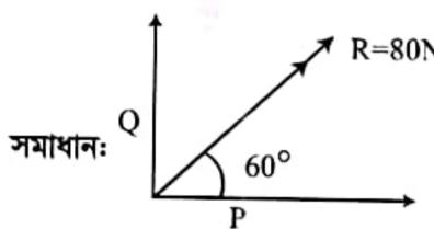
আবার, R  $\sin 60^{\circ} = P \sin 0^{\circ} + Q \sin 90^{\circ} \Rightarrow Q = 80 \sin 60^{\circ} = 40\sqrt{3} \text{ N (Ans.)}$
