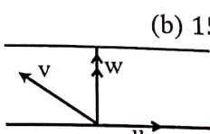
$$; v = \frac{100}{4} = 25 \text{ m / min}; w = \frac{100}{5} = 20 \text{ m / min}$$
